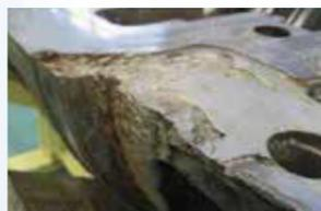
Erosion on inside of cylinder
