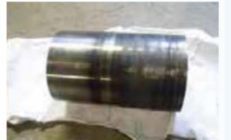
Shaft sleeve damage caused by gland packing seizure
