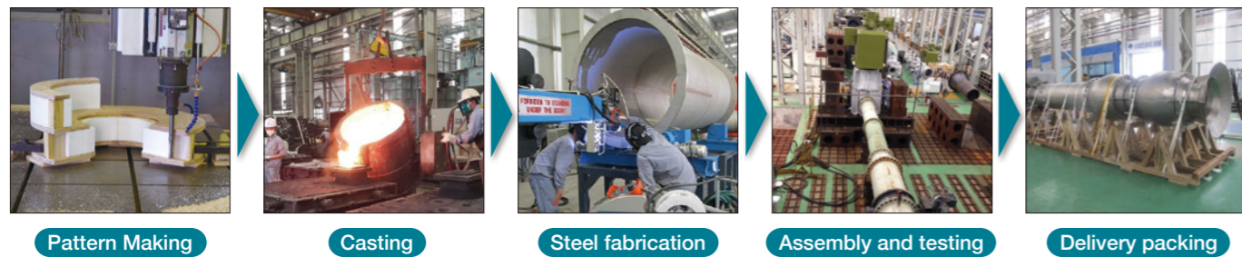
Ebara's factory is equipped with the necessary equipment, personnel and technology to perform all the main production processes in-house. This allows efficient control of production schedule and quality system to satisfy a wide range of Customer requirements and international standards.
