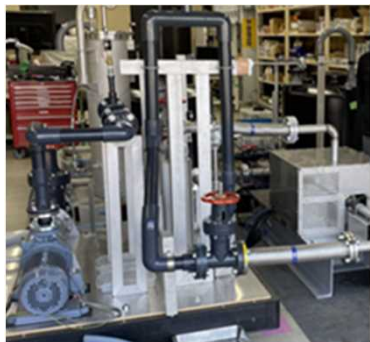
Testing equipment for components for turbo pumps (water-flow test) The photo provided by: Interstellar Technologies, Inc.
