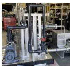
Testing equipment for components for turbo pumps (water-flow test) The photo, provided by: Interstellar Technologies, Inc.
