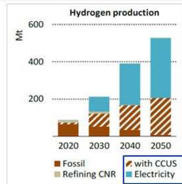
Figure 3.8 - Global production of hydrogen by fuel and hydrogen demand by sector in the NZE
