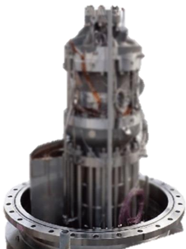
Picture of Liquid Hydrogen Booster Pump
