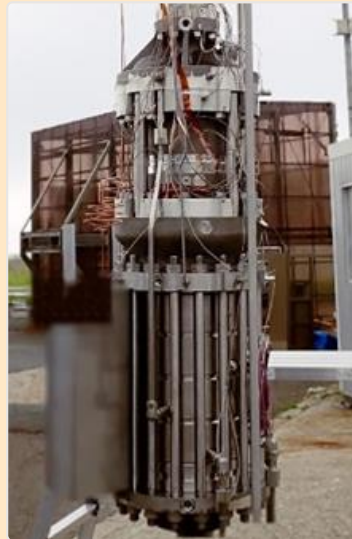
-253°C Liquid hydrogen centrifugal pump
