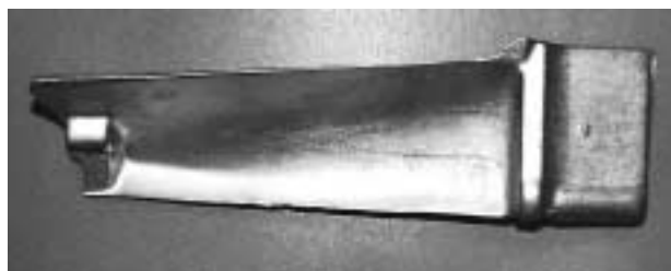
写真3 本開発合金製ガスエキスパンダ動翼 Photo 3 Appearance of the gas expander rotating blade made of the developed alloy
