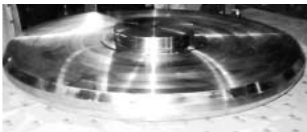
写真2 本開発合金製ガスエキスパンダディスク (φ1400 mm) Photo 2 Appearance of the φ1400 mm gas expander turbine disk made of the developed alloy
