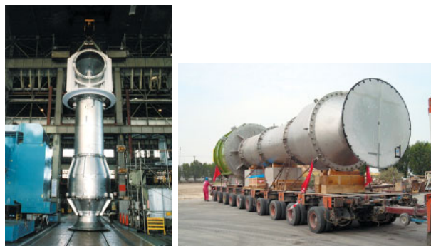
(a) 2相ステンレス鋼 (口径2000 mm) Duplex stainless steel (2000 mm nozzle diameter)
