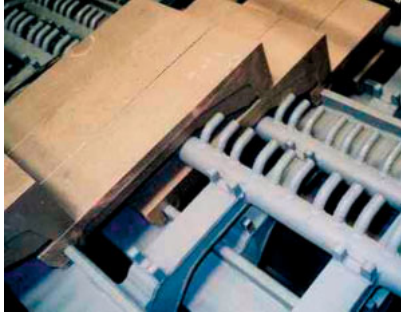
写真2 強制空冷火格子 Photo 2 Forced air-cooled type grate
