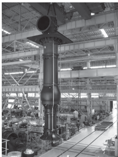
写真1 口径1500 mm立軸斜流ポンプ Photo 1 Vertical mixed-flow pump with 1500 mm bore
