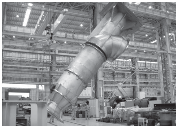
写真5 口径1800 mm 立軸斜流ポンプ Photo 5 Vertical mixed-flow pump with 1800 mm bore
